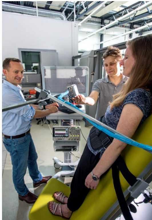
At the Innovation Campus Electronics and Microsensorics Cottbus (iCampus), a device is being developed that can measure respiration and heartbeat on a contactless basis. Via a secure data interface to the attending physician, this will later allow people in rural areas to also be monitored and provided with medical care, even if the medical practice is far away.
